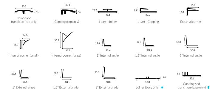
**Lengths:** 2440mm • 3050mm (Dimensions shown in mm)
