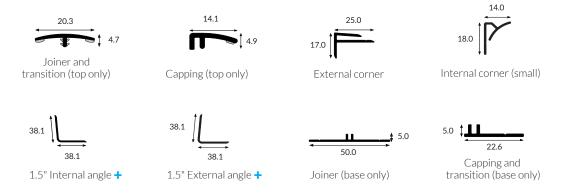
**Lengths:** 2500mm • 3050mm (Dimensions shown in mm)
