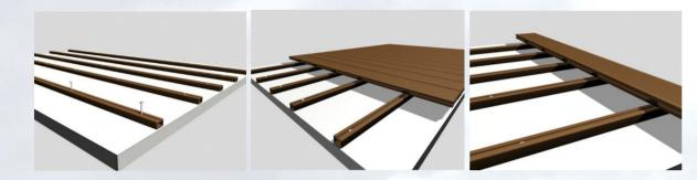
The WPC products' expansion rate is around 0.3% to 0.5% depends on different weather condition in different places, based on this expansion rate, there must always be a gap always between 2 WPC products, as follows:
