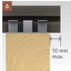
6 10 mm maximum board end overhang from joists.
