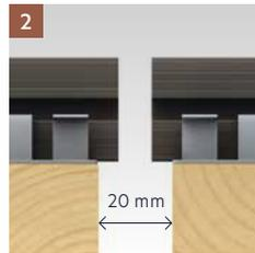
2 Double joists under butt joints, with one clip each side of the butt joint. Provide a 20 mm gap between joists.
