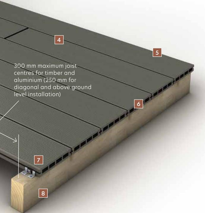
300 mm maximum joist centres for timber and aluminium (250 mm for diagonal and above ground level installation)
