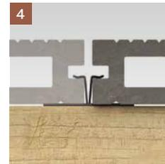
4 Composite Decking stainless steel fixing clips provide a secure fit and with the recommended 6 mm spacing of boards.
