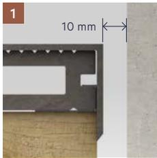
1 Provide a minimum 10 mm gap between edge of decking and any adjacent wall. Allow 8 mm gap if deck boards run parallel to a wall.
